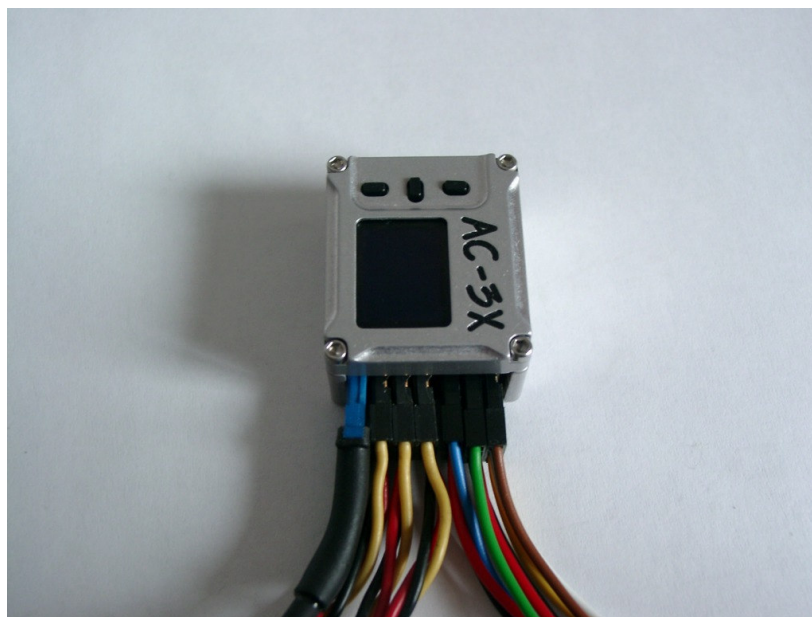
Figure 8: AC-3X with receiver wiring and 4 Servos connected
