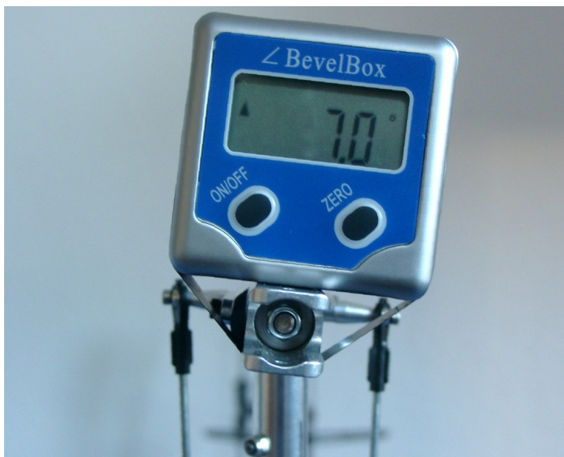
Figure 16: Cyclic angle of 7° at full swash stick input
