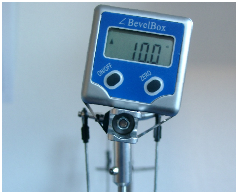
Figure 17: Full pitch, 10° on the blade grips
